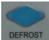
**Defrosting Indicator:** When the machine is defrosting, this indicator turns on. After defrosting, it turns off.
